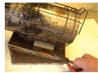
10. To do this remove the four nuts holding the smoker to the bellows. If they are rusty use some penetrating oil. Do not turn too hard on rusted nuts or you will strip the screws and then not be able to get them off.
