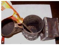
4. You do not have to get it perfect but remove the majority of the soot and carbon. Removing the crud from the can makes it easier to get the grate out in the next step.
