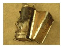
13. Check the bellows for leaks. To do this hold your finger over the air outlet hole and squeeze the bellows. Some air will leak but large leaks need to be fixed. Duct tape works as temporary fix but replacement with new one is best.
