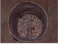
You may find debris and/or soot in the can under the grate. Scrape this and dump it out
