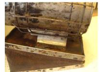
14. Replace the grate being careful to place a leg on either side of the inlet tube. Replace the bellows and tighten the 4 nuts. Putting a little oil on the threads makes the job easier next time.
